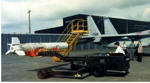
Figure 5. USAF Air-launched ASAT ASM-135A. Photo Taken at the Edwards AFB Flight Test Center
