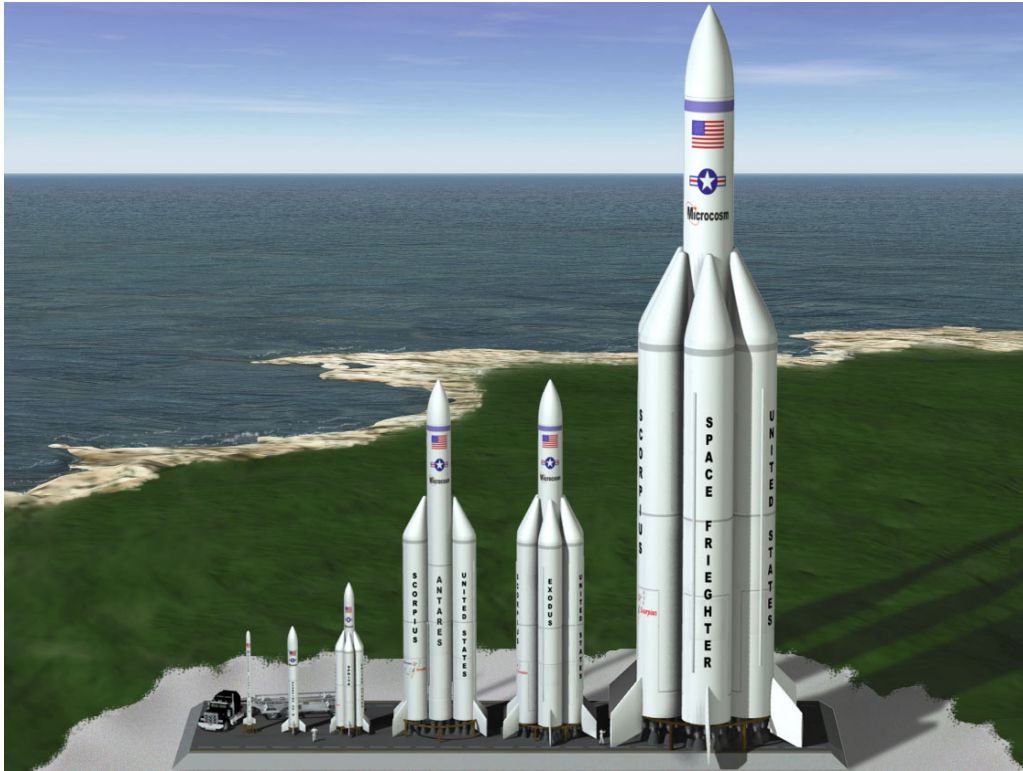
Fig. 1. The Scorpius® Family of Launch Vehicles. On the left, are the SR-S and SR-XM suborbitals and the Sprite Small Launch Vehicle. The intermediate-sized vehicles in the center are Antares and Exodus. The Heavy Lift Space Freighter is on the right.
