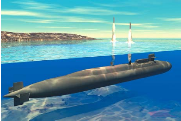
Artist Conception of a SSGN Tactical Trident outfitted to launch Tomahawks, UUVs, UAVs (U.S. Navy Image)
