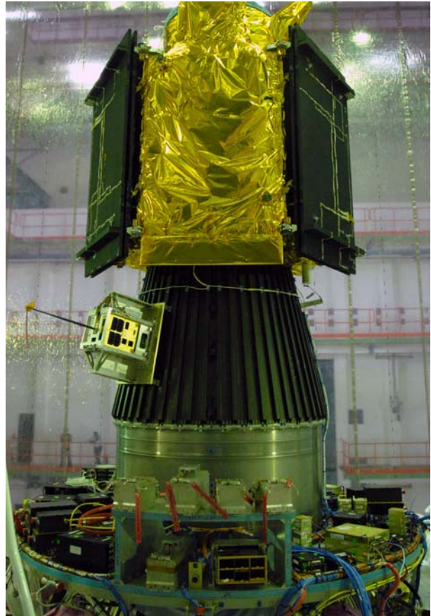
Figure 5. The PSLV-C9 upper stage showing NTS integrated on the XPOD GNB separation system mounted on the Payload Adapter cone.
