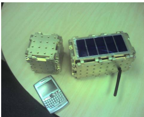
Figure 16. Concept satellites in the form of assembled nano-SPA based CubeSats. The left CubeSat is a 1U form factor, the right being a 2U form factor. The solar panels on the 2U are “mock”, and the protruding 802.11 antenna would not be suitable in an actual flight system.
