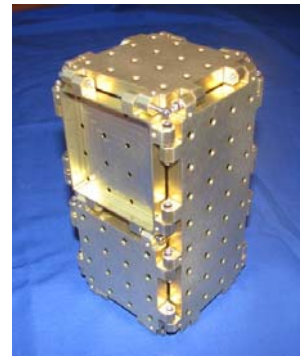
Figure 9. An example of a 2U cubesat (20 cm x 10 cm x 10 cm) based on a combination of 1×1 and 1×2 NMF facets.
