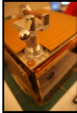
Figure 2 - Fixed boom holding the Langmuir Plasma probe and the Very Low Frequency Receiver antenna in the background.
