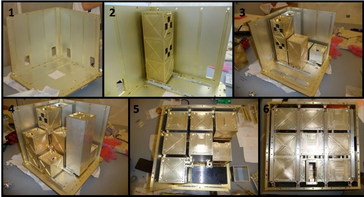
Figure 4 – Assembly of the BUSAT spacecraft starting with the primary structure and then the filling of the subsystem cubes.
